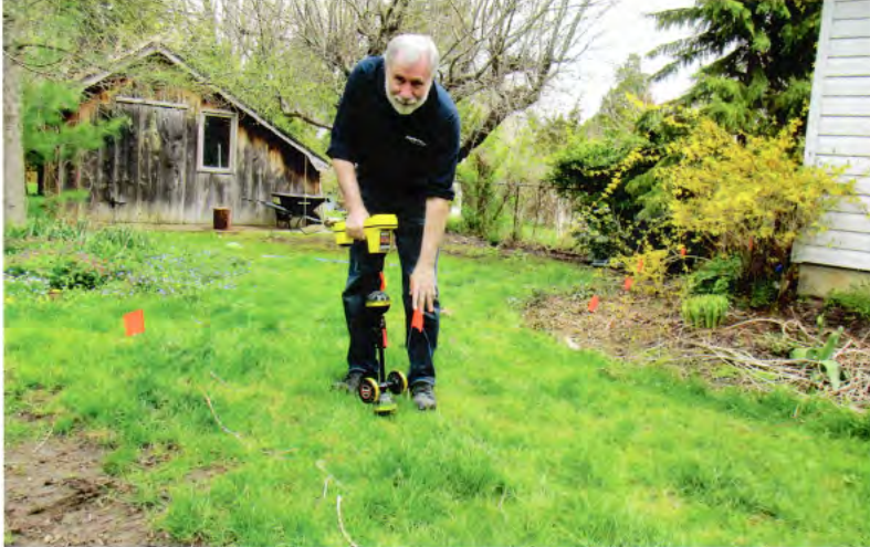
A locator is used to read the signal being transmitted by the camera below ground at one suspect leak location in the lawn area.
